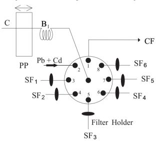
**Figure 1.** Automated experimental setup:  $SF_1$  to  $SF_3$  (sample flasks) containing metal solution in contact with meat submitted to renewed aliquot volume after 1 h, during 8 h;  $SF_4$  to  $SF_6$  containing metal solution in contact with 1 g of meat, during 8 h; PP (Peristaltic Pump); C (Carrier-deionised water); B<sub>1</sub> (Holding Coil) and CF (Collection Flask).
